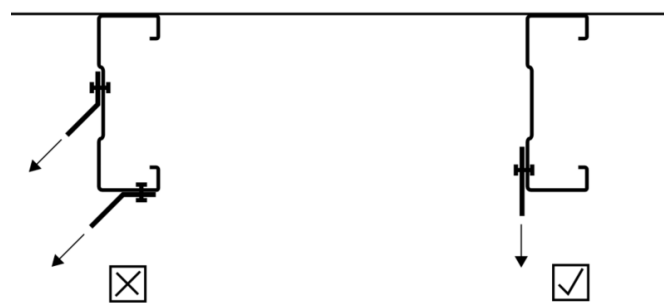
Figure 17: Connecting seismic restraint braces to light gauge purlins
