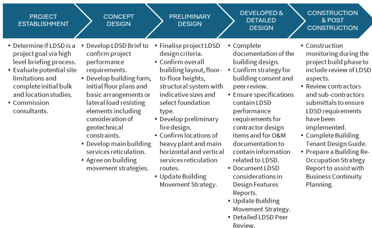
Figure 2-1 Recommended LDSD design process
